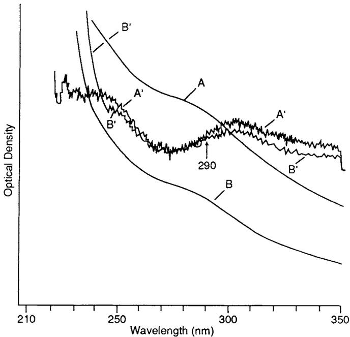
FIG 6.4 Absorption spectra of dopamine melanin (A) and *substantia nigra* melanin (B) solubilized in sodium borohydride. A' and B' represent the first derivative spectra of A and B respectively.
