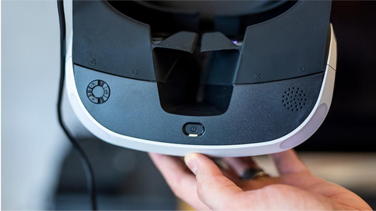
1. Press the activation button at the bottom of your VR headset. The tracking lights on the back will light up blue.
